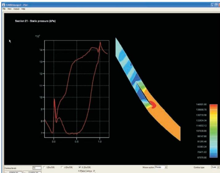
2D view of the blade pressure distribution and blade to blade contours.
