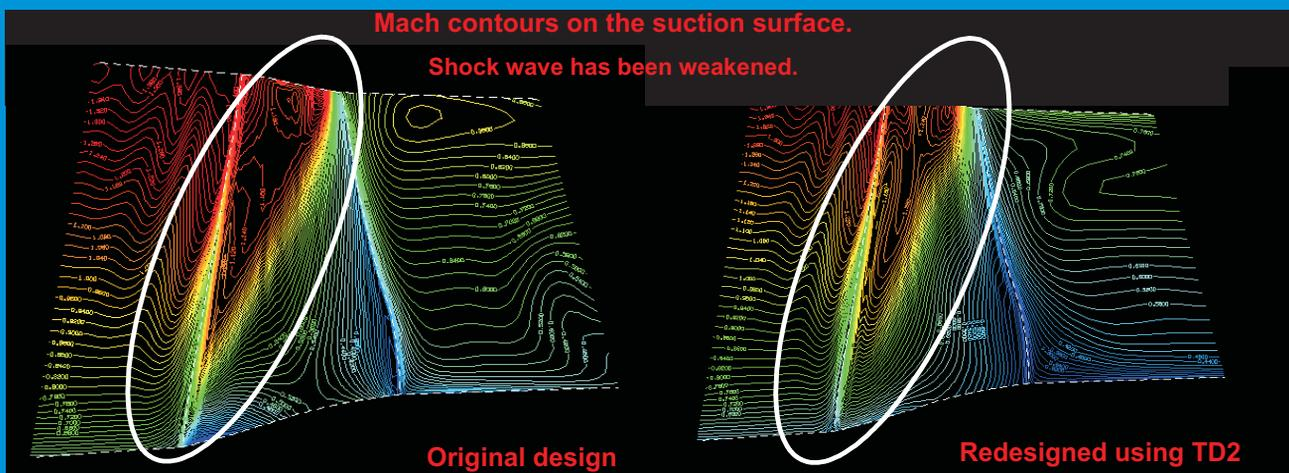
Comparison of Mach number distribution near the suction surface of the original NASA 67 rotor with the rotor designed by TURBOdesign-2 indicates considerable reduction in the preshock Mach number in the designed Rotor.
