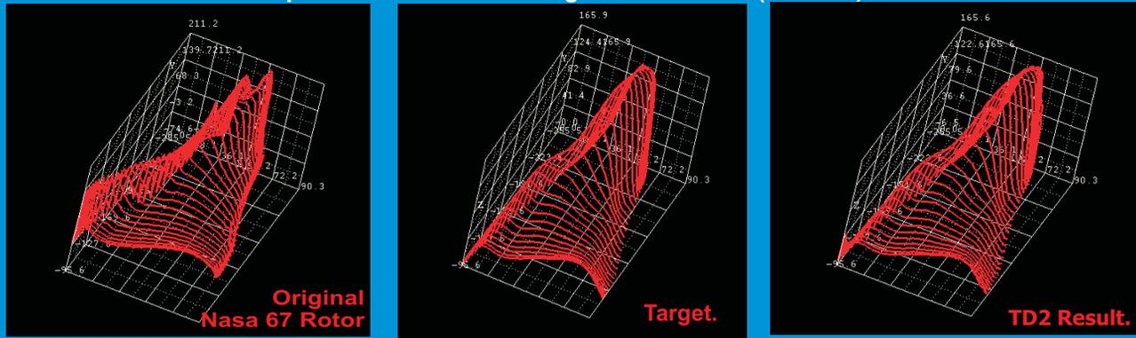
TURBOdesign-2 inverse design method with the multigrid technique is robust and fast. Typical CPU time needed on a Pentium 4 2.0 Ghz is about 1.3 hours, which will depend on the difference between target  $\Delta P$  distribution and the original one. The blade loading can be easily and interactively modified by using B-spline control on as many or as few sections required. Smooth blade geometry usually can be obtained from the redesign, as long as the loading distribution is smooth.
