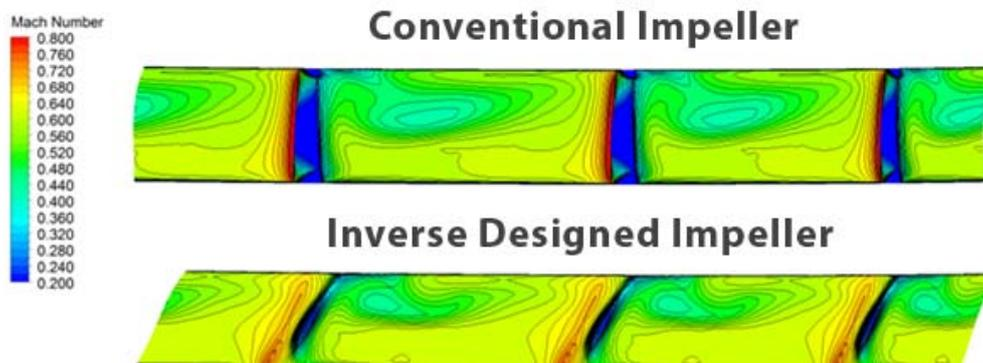
Image 4. Comparison of Exit Relative Mach Number between the Conventional impeller and the Inverse design Impeller showing reduction in exit flow non-uniformity
