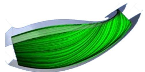
Image 2. Secondary flows on the suction surface of the original impeller
